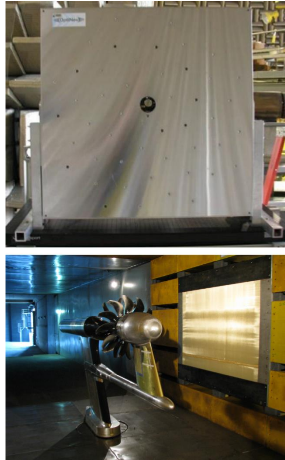
Figure 3. The Array48 system and its installation in the wall of the wind tunnel [15]
